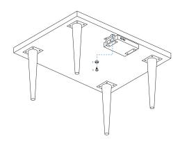
Use the four provided No. 6 screws ("D") and the four cup washers ("E") as shown in the diagram to the left to secure the gadget to the plywood underside of the counter, desk, or table.
