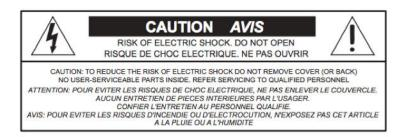
Chameleon audio processors have an internal 120VAC / 240VAC power supply. Hazardous voltages are present whenever the unit is plugged in and may still be present on certain components even when the unit is unplugged.
