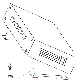
Use the four provided No. 6 screws ("E") and cup washers ("F") as shown in the diagram above to secure the gadget to a plywood surface.
