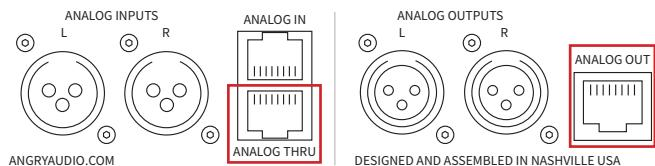
The Analog section of the rear panel hosts two items to take note of. The ANALOG THRU connector is useful for daisy chaining the same input source to multiple devices. The ANALOG OUT StudioHub+ RJ-45 connector provides audio and ±15VDC to certain types of connected devices.
