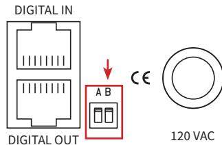
Find the DIP switches on the rear panel, adjacent to the line cord. For ANALOG input, leave DIP switch B in the "down" position. To select DIGITAL input, flip DIP switch B to the "up" position.
