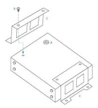
Use the four provided No. 6 screws ("D") and the four cup washers ("E") as shown in the diagram to the left to secure the Gadget to the plywood underside of the counter, desk, or table.
