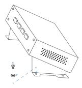
Use the four provided No. 6 screws ("E") and cup washers ("F") as shown in the diagram above to secure the Gadget to a plywood surface.
