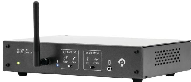
Once paired, it negotiates the optimal codec algorithm (usually APT-X for Android and AAC for iOS) and connects to your console using analog I/O on balanced XLR jacks. The sound quality is top-notch, and because the Bluetooth Gadget is bi-directional, callers are provided with a mix-minus feed. Most broadcasters will be familiar with the concept of mix-minus, but for our podcaster friends or live and studio sound engineers, here’s a resource you may find helpful:
