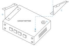
Use the four provided No. 6 screws ("E") and cup washers ("F") as shown in the diagram above to secure the gadget to a plywood surface.
