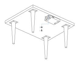
Use the four provided No. 6 screws ("D") and the four cup washers ("E") as shown in the diagram to the left to secure the gadget to the plywood underside of the counter, desk, or table.
